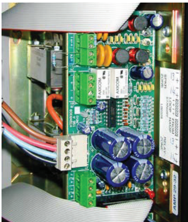
PA0691 HTRN9308-1 2x50W Transformer Module
