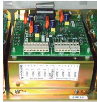
PA0795 TRAN9706-1 4x10W Transformer Module without Relays
